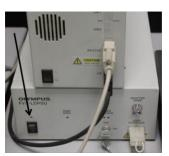
Multiline Argon laser (458,488 and 515 nm) for CFP, GFP, YFP, CY2,FITC, etc.
