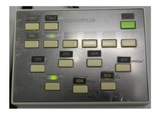
**6**. If you will use x40 or x60 water immersion objectives , do not forget drop water from universal vial (one drop !!!).
